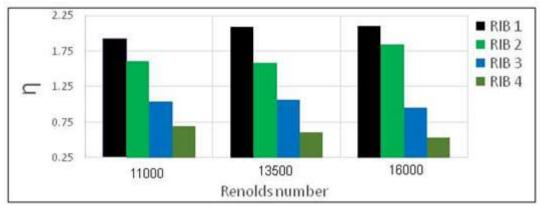
Figure (13): Enhancement factor as a function of Reynolds number
