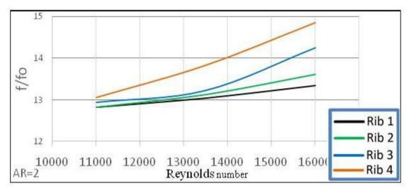
Figure (12): Friction factor ratio variation with Reynolds number for different rib configuration and AR=2
