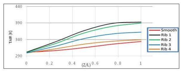
Figure (9): Air temperature distribution at the channel centerline for (Re=16000) and AR=2
