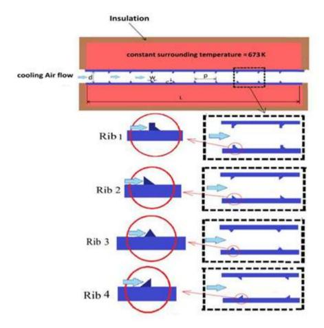
Figure (7): Location of ribs inside the channel
