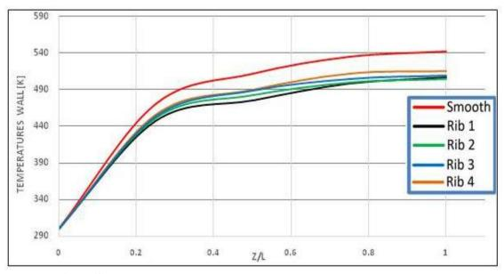
Figure (8): Temperature distribution for the inner wall surface channel with AR=2
