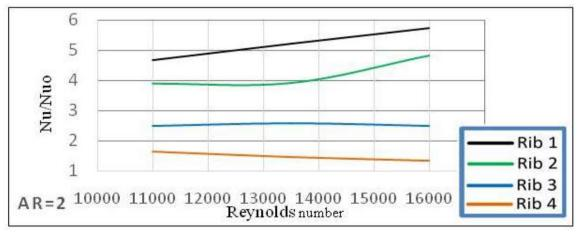
Figure (11) Normalized Nusselt number as a function of Reynolds number for AR=2
